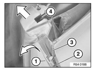
Unclip finisher strip (1) until guide (2) leaves the mucket (3) and remove the mucket.
