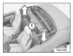
Press down convertible top (1) on one side of main bearing with second person lifting opposite side at the same time, thus lifting convertible top out of its compartment.
