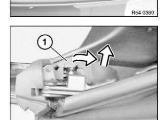
Lift right trim piece (1) out of the main bearing threading toward the rear and pull out upward.
