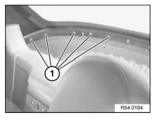
Screw in all remaining screws (1) on left/right sides and tighten down.
