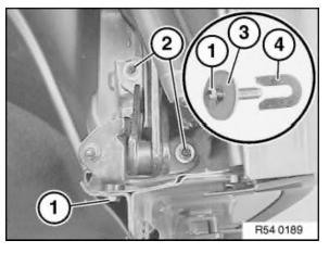
Unfasten left/right screw (1) and nut (2). Remove screw (1) with washer (3) and shim (4).
