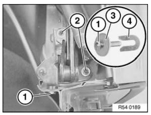
If the convertible top does not fit in longitudinal direction, change the number of shims (4) in longitudinal direction.
